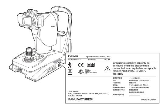
The position and contents of the label attached on the CR-2 is shown below. Follow the information on the label to use the CR-2 appropriately.
